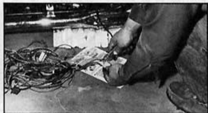
LEFT —Drill a hole in the electrical component bracket and mount the whole assembly and electrical box on engine bolts.
