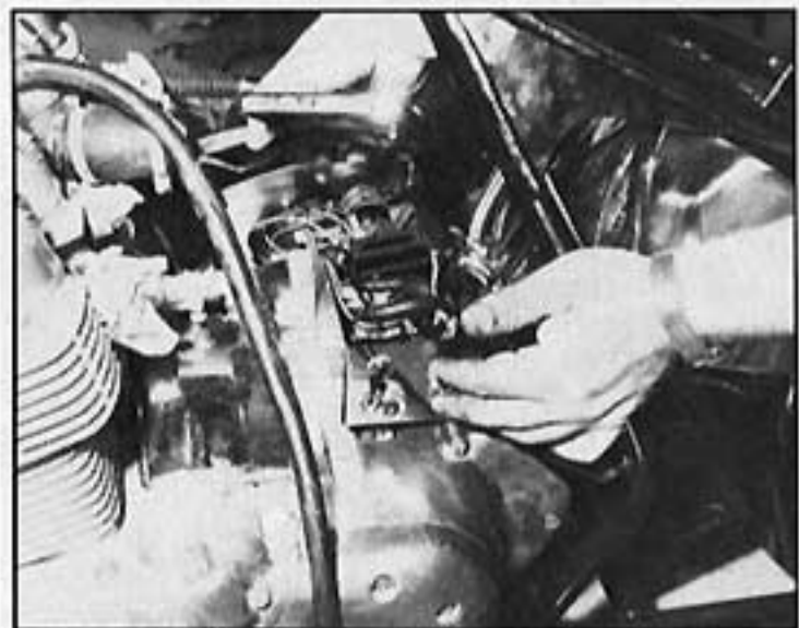
ABOVE—A large cable-like wire coming out of the starter motor must be connected to the B. terminal of the solenoid.
