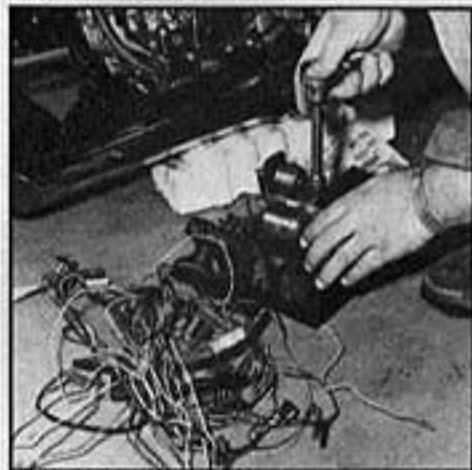
ABOVE—The Honda 750 electrical components are mounted onto a bracket which is mounted onto the stock battery box.
