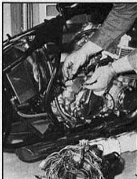
All of the stock wiring must be removed from the motorcycle. You will be left with a bundle of wire beside the bike and two sets of wires coming out of the engine.
