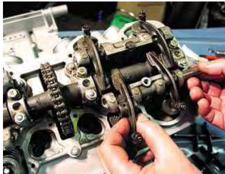
2: This sohc Honda engine uses only one camshaft, and has rocker arms to transfer the cam movement to the valve stems. Note the screw and locknut adjusters, which make it easier to set up for wider cam profiles.
