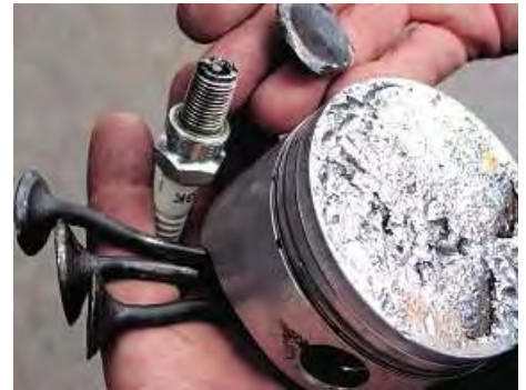
3: When it all goes wrong. This drag-race GSX engine lost a valve head when the valves hit the piston crown. Check you have the correct clearances before running an engine with high lift cams.
