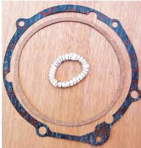
2. Three different types of gasket from the set: asbestos for the exhaust, cork for the contact breaker points cover and asbestos/rubber for an outer case.
