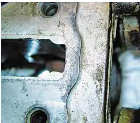
4. The camchain tunnel has this rather narrow joint face: a thin smear of sealant will help the gasket stay oil tight.
