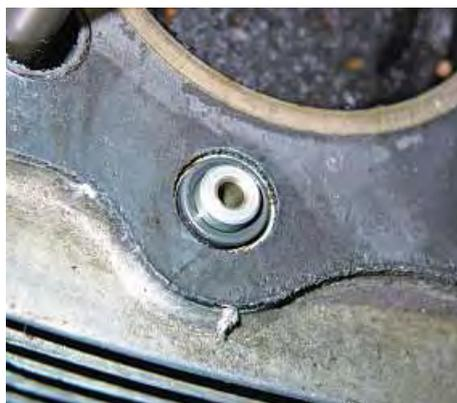
5. This oil restrictor jet should be sealed adequately by its surrounding O-ring.
