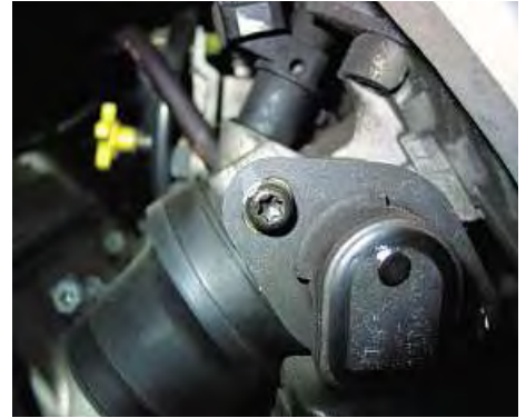
Another type of head used on modern bikes, this is Torx on a fuel injection component – in a way an up-to-date version of Picture 4. I am quite keen on these as they provide a very positive and slip-proof drive.
