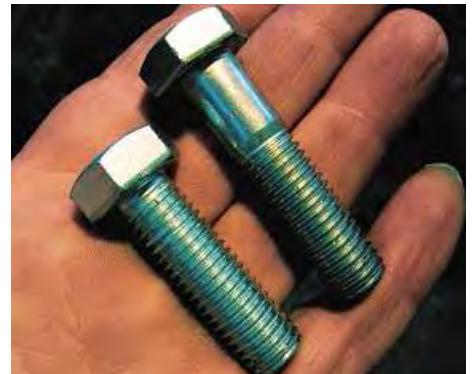
The word 'bolt' is widely misused: the uppermost fastener is one, the other is not – it is a setscrew.
