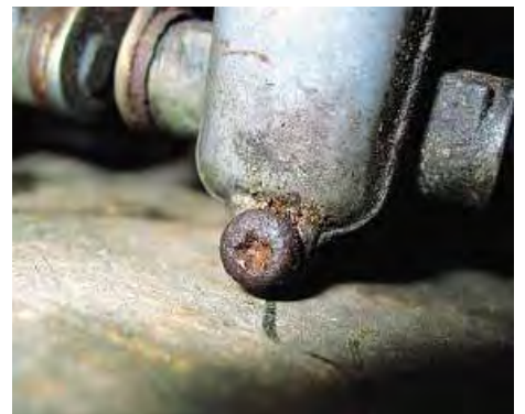
A typical Phillips-headed setscrew, this on a carburettor top. So convenient for the factory to fit, but often so inconvenient to remove thirty years later.
