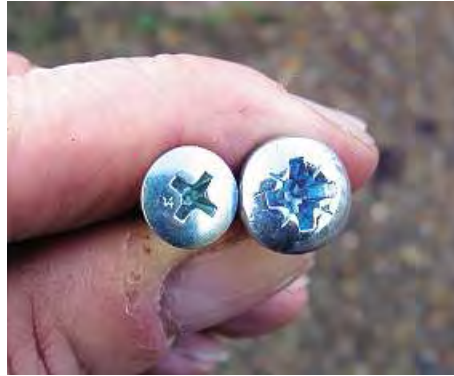
Here we see a comparison between Phillips (left) and Prodrive heads. The latter is much less likely to slip. You might be able to see a tiny cross on the Phillips fastener; this indicates that the thread form is ISO not JIS.
