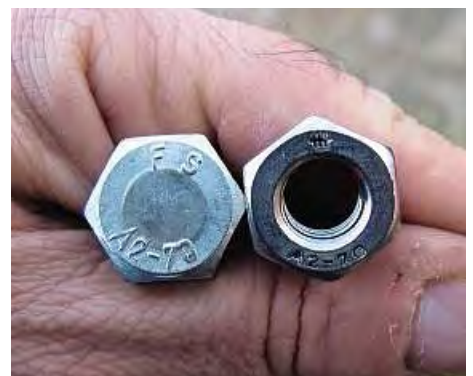
The A2 on these components tells us that they are stainless steel. Attractive, corrosion-proof and really not too expensive at around twice the price of BZP fasteners.
