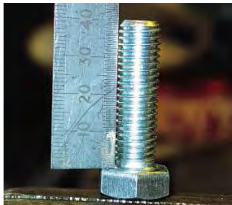
This is how to measure the length of a setscrew: from the extreme point of the thread to under the head.
