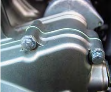
Phillips heads have mostly been replaced these days. This is a modern crankcase cover, held on with ordinary hex-headed setscrews.
